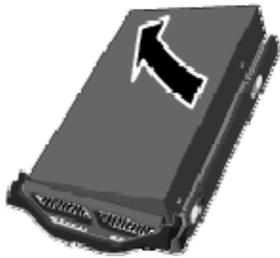
9. Fold up the flap near the back of the hard drive tray.
