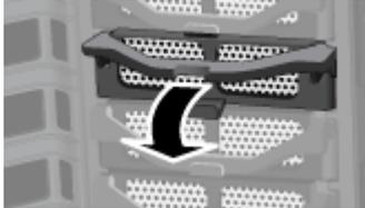
5. Using a coin, turn the security knob counterclockwise to lock system drive in its bay.
