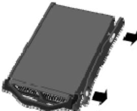
8. Flex the front of the right side-rail and withdraw the front pin from the hard drive by gently pulling the side-rail down and away.
