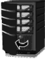
3. Using a coin, turn the security knob clockwise to unlock the drive.
