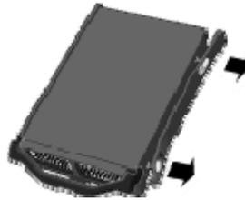
7. Flex the front of the right side-rail, and then withdraw the front pin from the hard drive by gently pulling the side-rail down and away.
