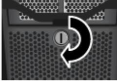
4. On the bottom drive, press down the lever to release the handle.
