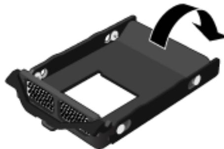
**Note:** This flap improves air flow through the server. If you remove a drive, be sure to fold this flap back up.
